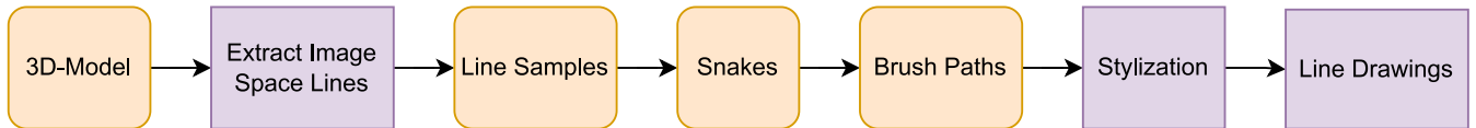
Figure 3: Active Strokes pipeline. Orange boxes with rounded corners are computed on the CPU while purple boxes with square corners are computed on the GPU. The uncertainty information is passed from the 3D model to the brush paths. It can then be used in the stylization step to create varying line styles depending on the uncertainty at a particular position.
